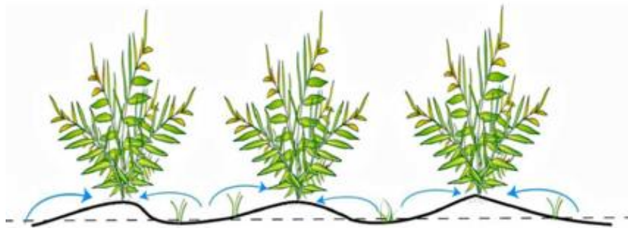
Figure 5. Sediment is preferentially eroded from bare and grass sites and deposited under shrub sites via canopy trapping ( Ravi et al. , 2007).
