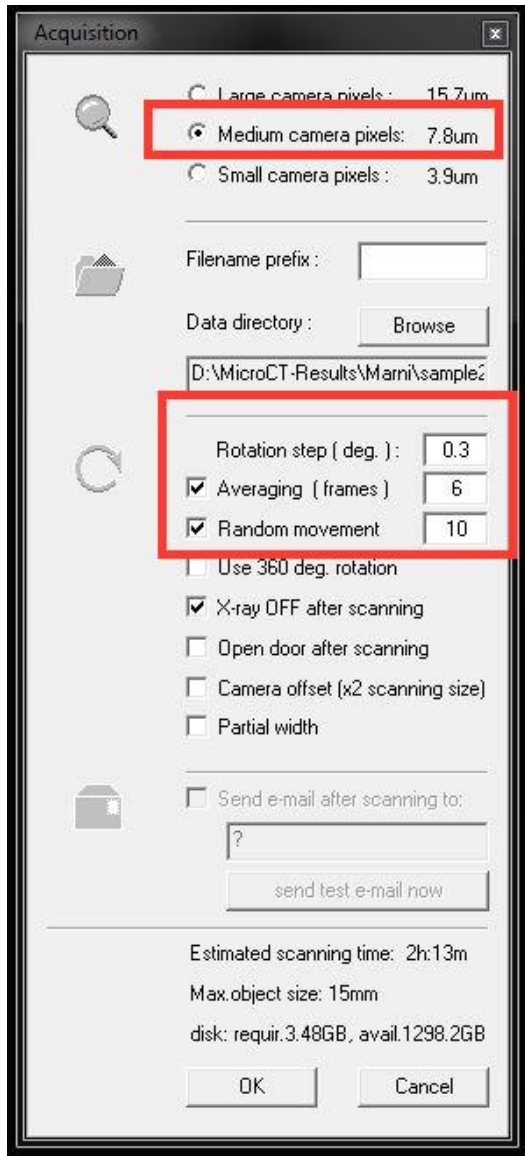
Figure 5: 0.3 degrees of rotation, frame averaging of 6, random movement 10
