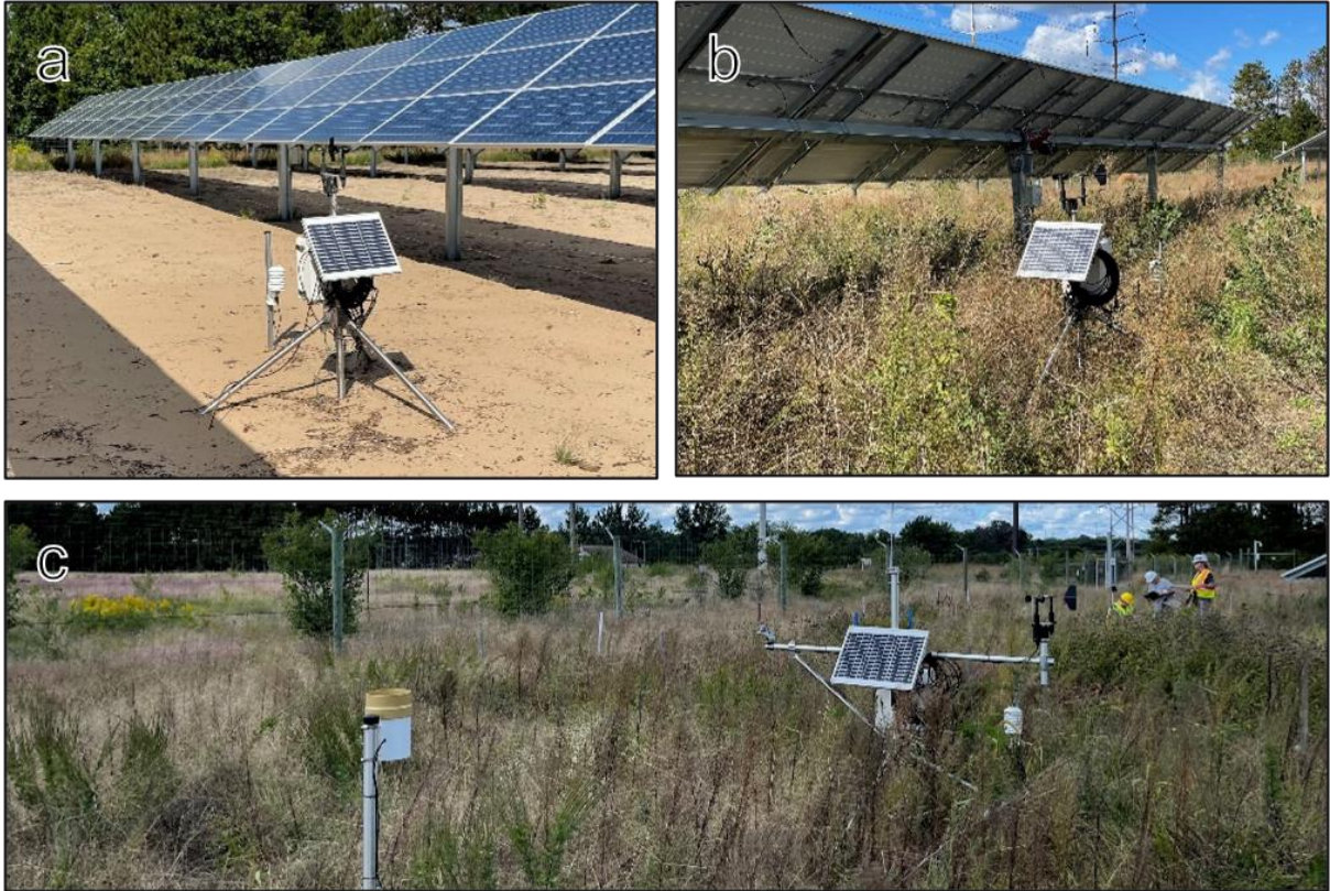
Figure A.2 Sensor towers in a. bare PV treatment; b. veg PV treatment; and c. Control.
