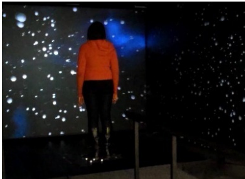
Figure 3.2-1. The three-wall virtual environment (CAVE) with virtual images of random size spheres on a black background projected on the three screens (front, left and right). Subject is standing on the dual force plates.
