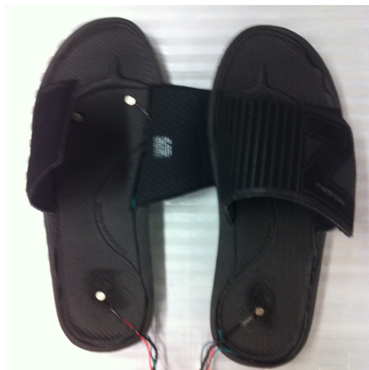
Figure 3.1-2. Open-type footwear (flip-flops) with the embedded vibrator motors on the heel and two on the metatarsal phalangeal joint.
