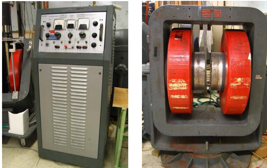
Figure 3.1. Magnion Power Supply and Magnet. The model number of the power supply is HS-1365B (left). The system is able to provide a uniform magnetic field of 1.5 Tesla between the poles.
