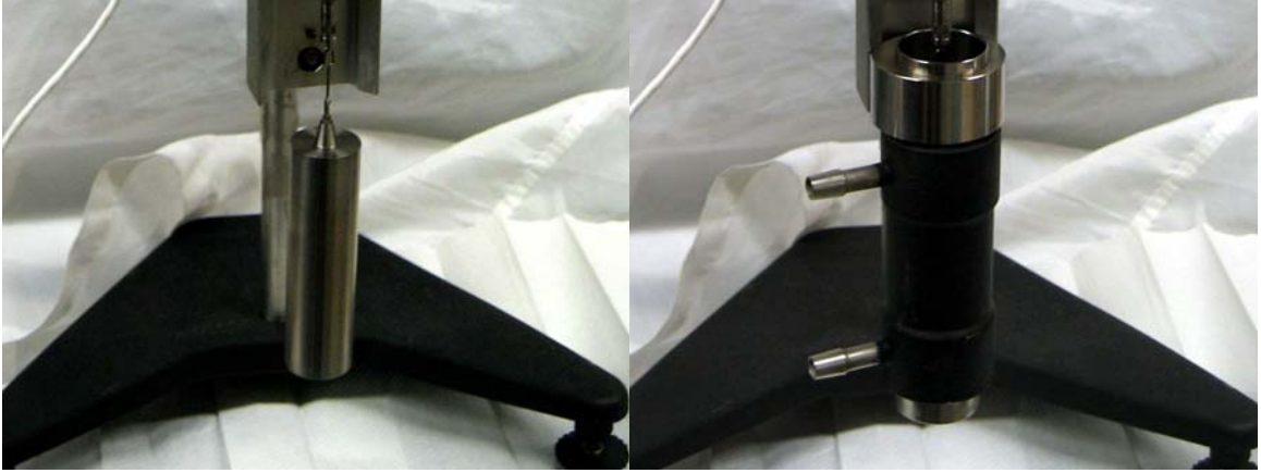
Figure 3.6. Spindles Used in Viscosity Measurements II. The ULA Spindle is shown in the left picture, and its container and water jacket are shown on the right.
