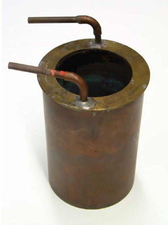
Figure 3.18. Container with Water Jacket.
