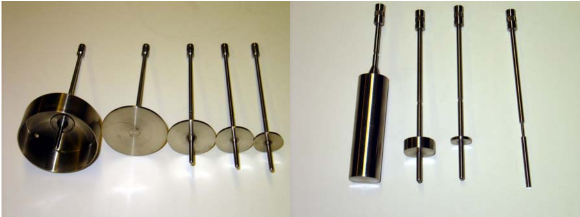
Figure 3.5. Spindles Used in Viscosity Measurements I. Spindles in the left picture are HA/HB-1 to HA/HB-5, and spindles in the right picture are LV-1 to LV-4.
