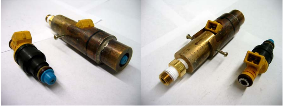
Figure 3.14. Fuel Injector and the Adapter. In the right picture it can be seen that the fuel injector has two control taps, which respond to an electric pulse and open the injector for the duration of the pulse.
