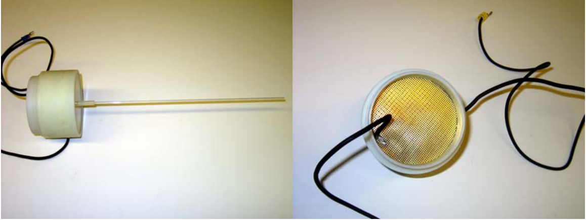
Figure 3.10. Mesh Capacitor Sample Treatment Container. The left picture shows a device of this kind with a glass tube and an adapter mounted on the bottom plate. The top mesh with lead soldered on it is shown in the right picture.
