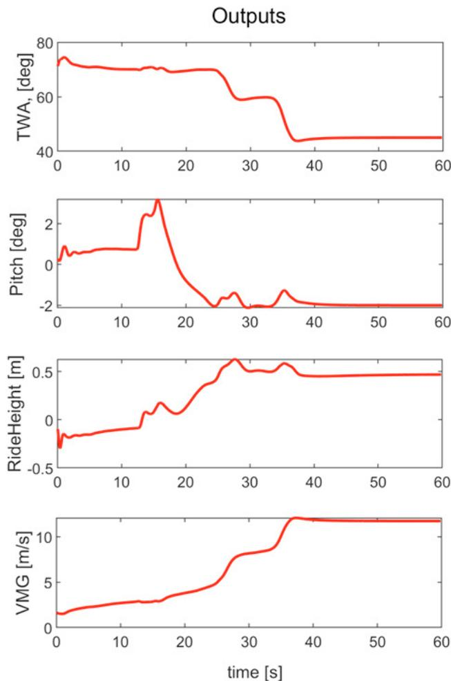
Fig. 4. Optimal outputs of the takeoff maneuver
