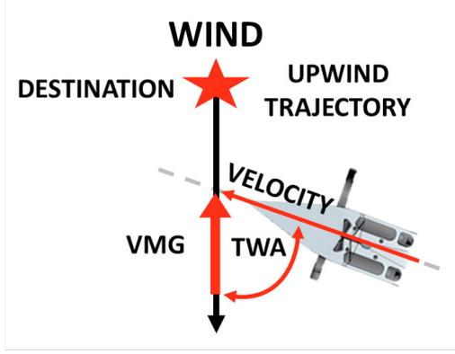
Fig. 1. Depiction of sailing metrics for an upwind trajectory
