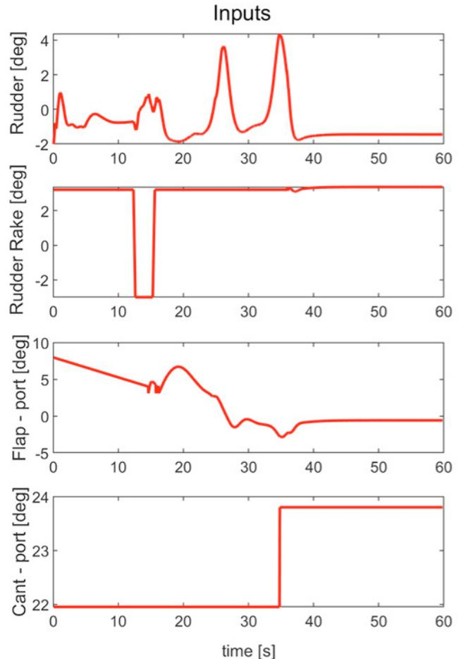
Fig. 3. Optimal inputs of the takeoff maneuver
