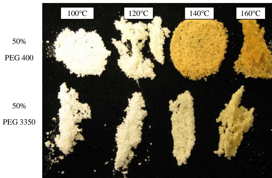
Figure 33. PVAP Mixtures Containing 50% PEG 400 or PEG 3350 and Heated to 100°C, 120°C, 140°C and 160°C
