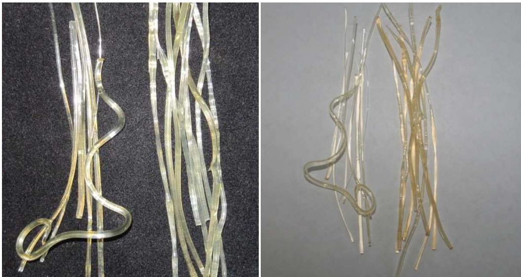
Figure 45. Extrudate Containing ITZ-PVPVA and ITZ-PVAP-PVPVA on a Black (Left) and White (Right) Background
