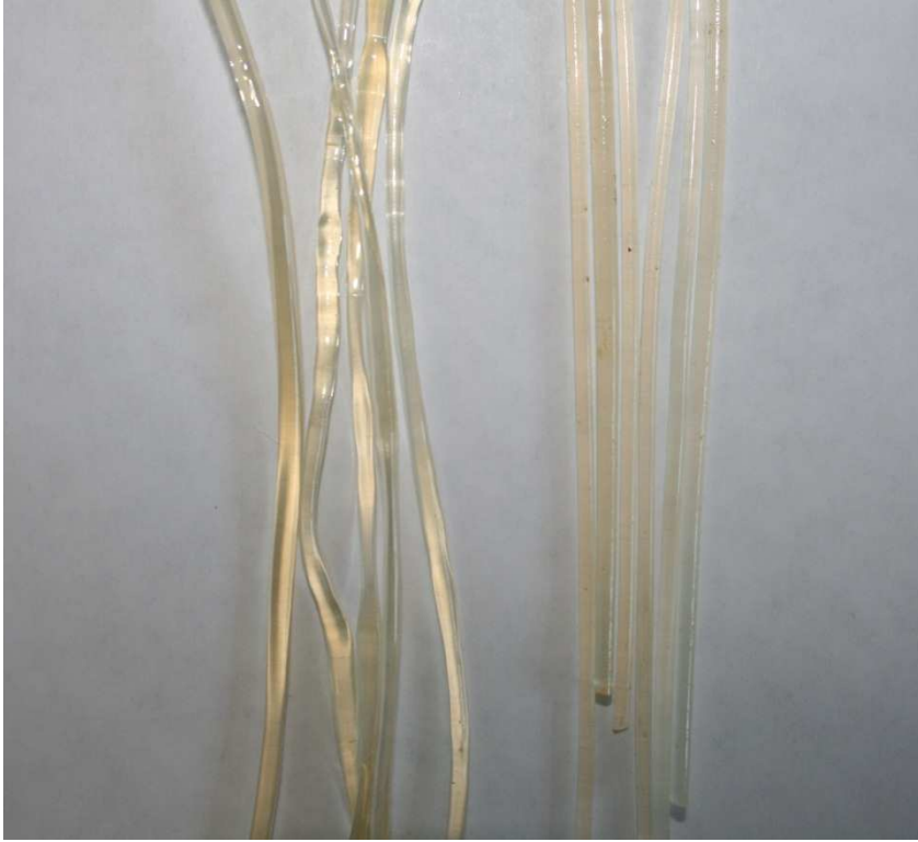
Figure 53. Extruded ITZ-PVAP-PVPVA (left) and ITZ-PVPVA (right) Solid Dispersions After 6 Months of Storage at 30°C/65%RH
