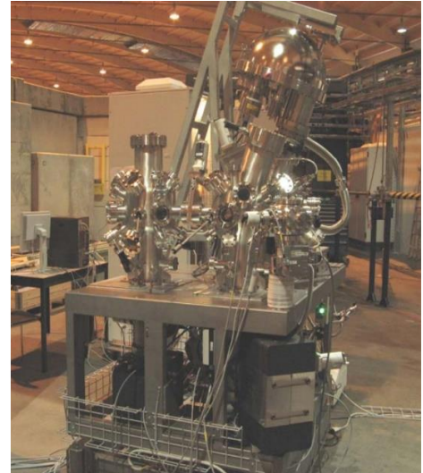
Figure (2.2) SX-ARPES endstation at the ADDRESS beamline of the SLS (adopted from reference [10]).
