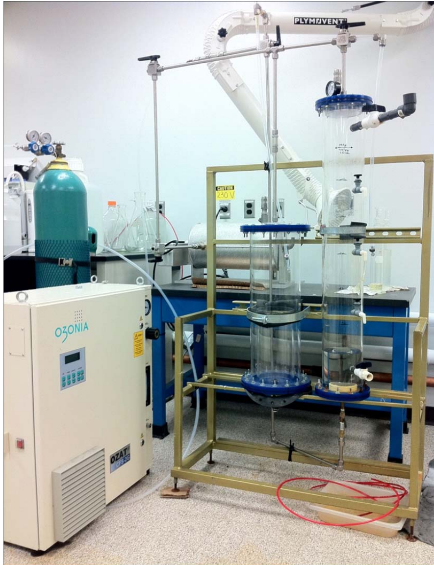
Figure A.1: Semi batch ozone reactor setup
