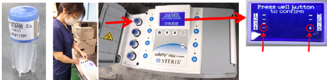
Figure 2. Processing of autoclaved Steris Celerity 20 Steam Biological Indicator (left). After 20-minute incubation in Celerity Steam incubator (center), fluorescent \alpha -glucosidase levels were spectrophotometrically evaluated, with increased fluorescence (+ sign) indicating failed sterilization, and no change in fluorescence (- sign) associated with successful sterilization (right).
