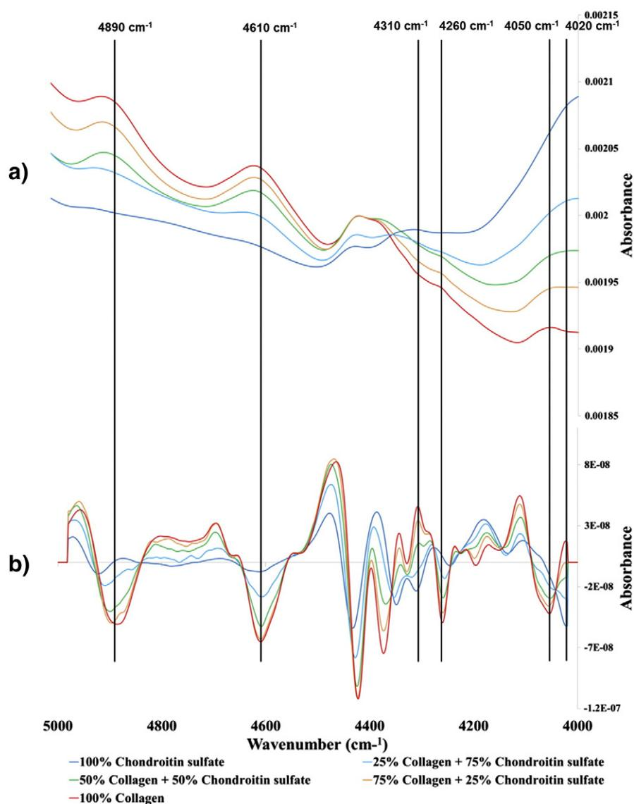
**Fig. 1.** The average scatter corrected and normalized (a) and second derivative spectra (b) of KBr pellet mixtures of collagen and chondroitin sulfate. Vertical lines indicate peaks of interest.
