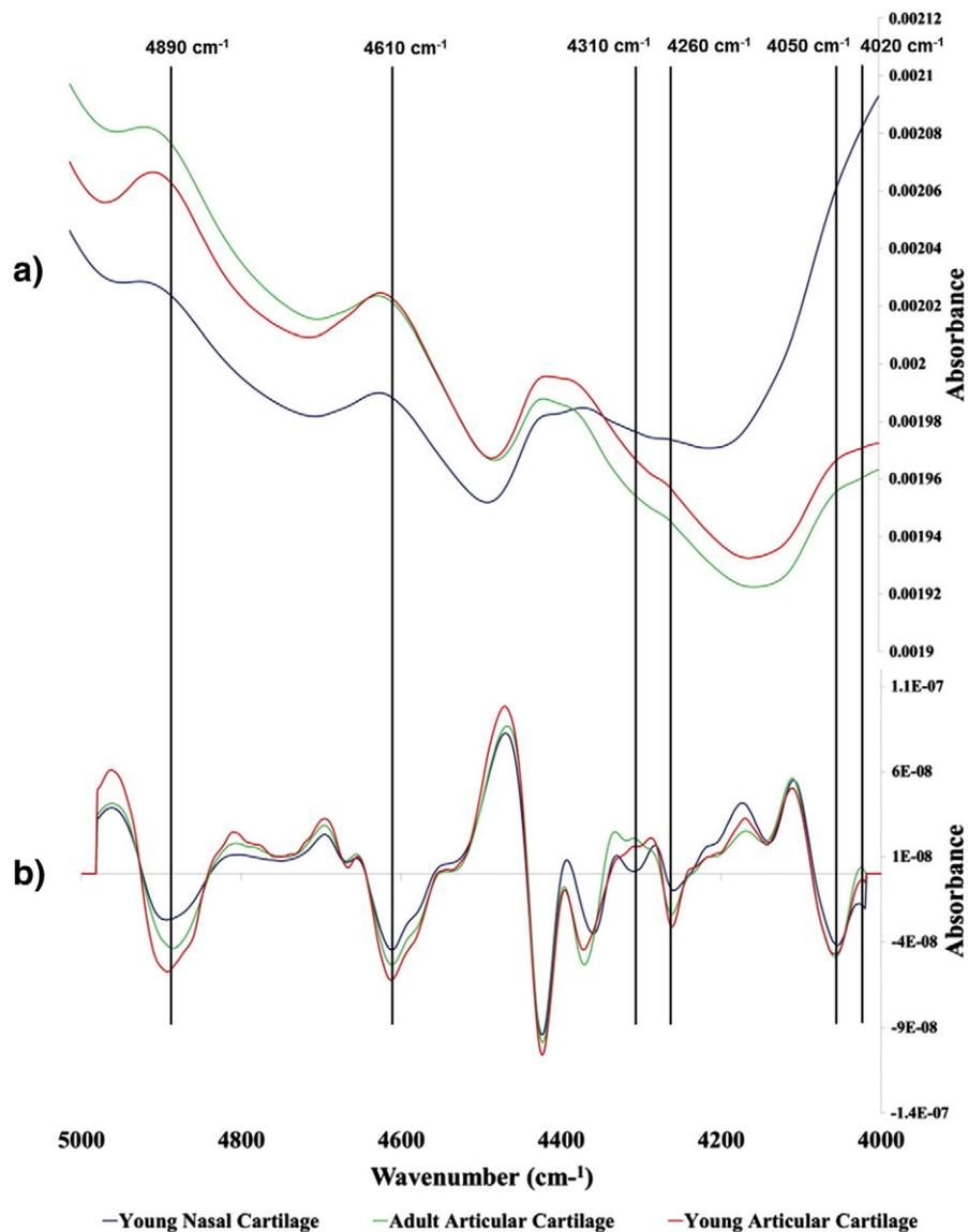
Fig. 2. The average scatter corrected (a) and second derivative spectra (b) of articular cartilage and nasal cartilage powders. Vertical lines indicate peaks of interest.
