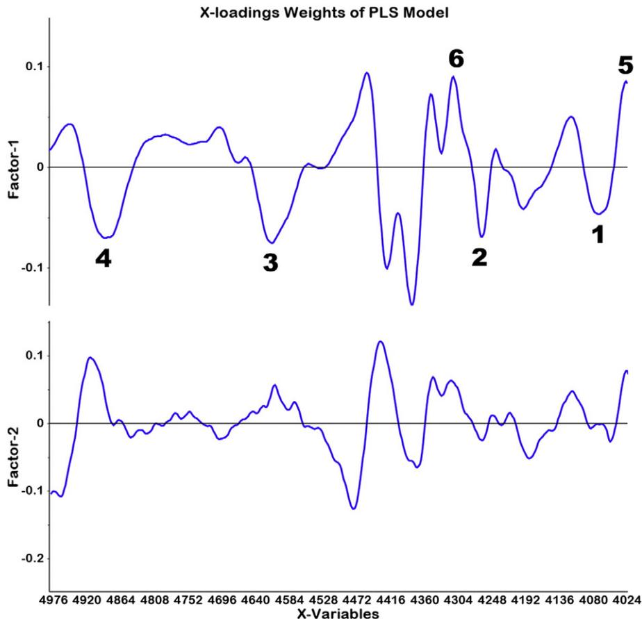
**Fig. 4.** The weights for the X-loadings used in the PLS model for estimation of collagen in pellet samples. Peaks of interest related to pure collagen spectrum (1–4) and chondroitin sulfate (5–6). Since a binary system was used for building the PLS model, the loadings for estimation of chondroitin sulfate percentage are inverse and hence not shown.
