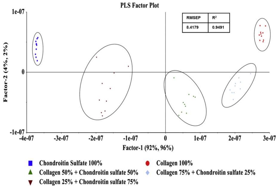
**Fig. 3.** The first versus second factor plot of the PLS model of collagen and chondroitin sulfate KBr pellet mixtures illustrating the pellet sample groupings based on varying collagen percentages.
