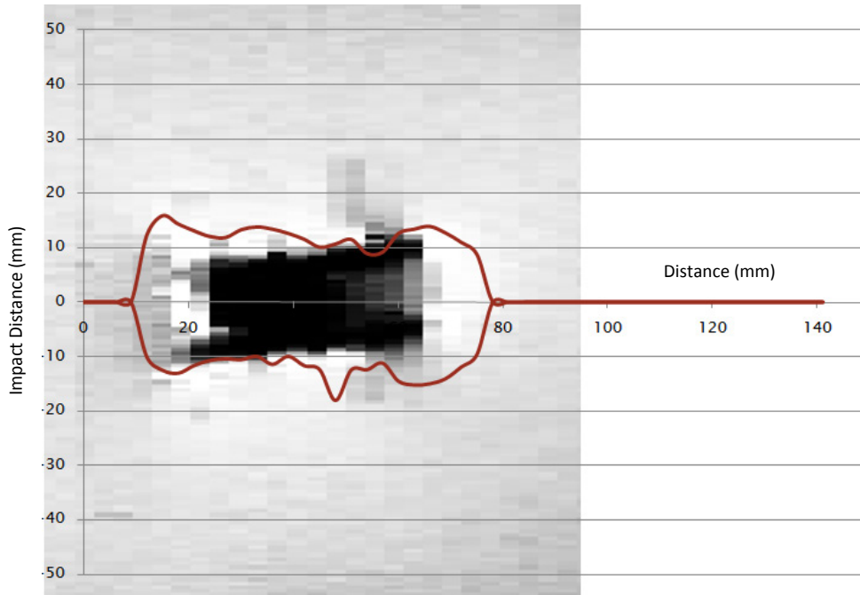
Figure 16 – Impact distance vs. distance (in mm) along titanium mesh cage axis superimposed over T2 TSE image of phantom.
