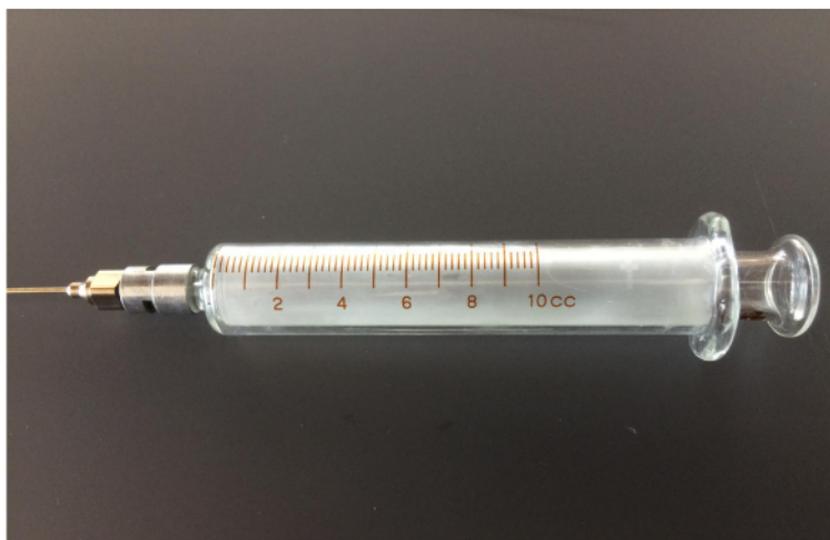
Figure 2: The Syringe with Needle. A 10 ml syringe with a needle attached using a Luer-lock tip is shown. Please click here to view a larger version of this figure.
