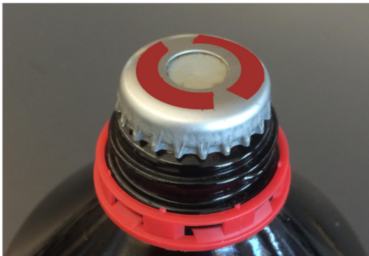
Figure 3: Septum-sealed Bottle Cap. The reagent is sold by the vendor with a sealed metal bottle cap with a rubber septum that may be pierced with a needle. Please click here to view a larger version of this figure.
