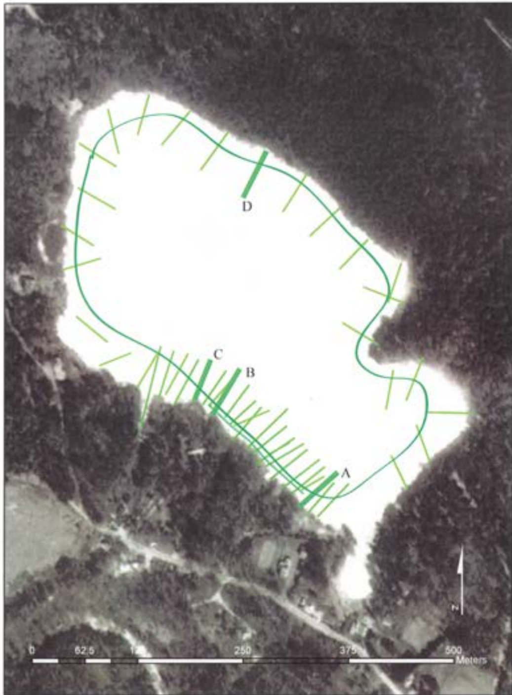
Figure 3-12. Location of Radar Surveys at Mirror Lake. ~50 m GPR transects were conducted at 50 m intervals around Mirror Lake. Transects were conducted at approximately 10 m intervals along the southwest shore. Two parallel-to-shore surveys were conducted: one about the perimeter of the lake and one along the southwest shore. Lines (A), (B), (C), and (D) are discussed in the Results Chapter.
