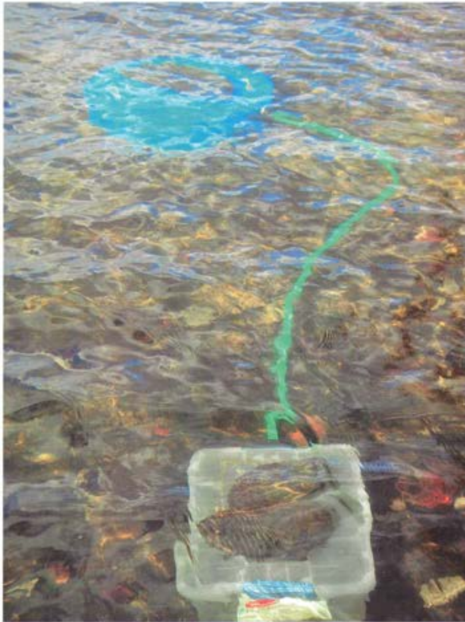
Figure 3-13. Seepage Meter. Seepage Meter (blue cylinder) attached to measuring bag, which is protected from waves and wind by the clear plastic case and held in place by a large rock (foreground).
