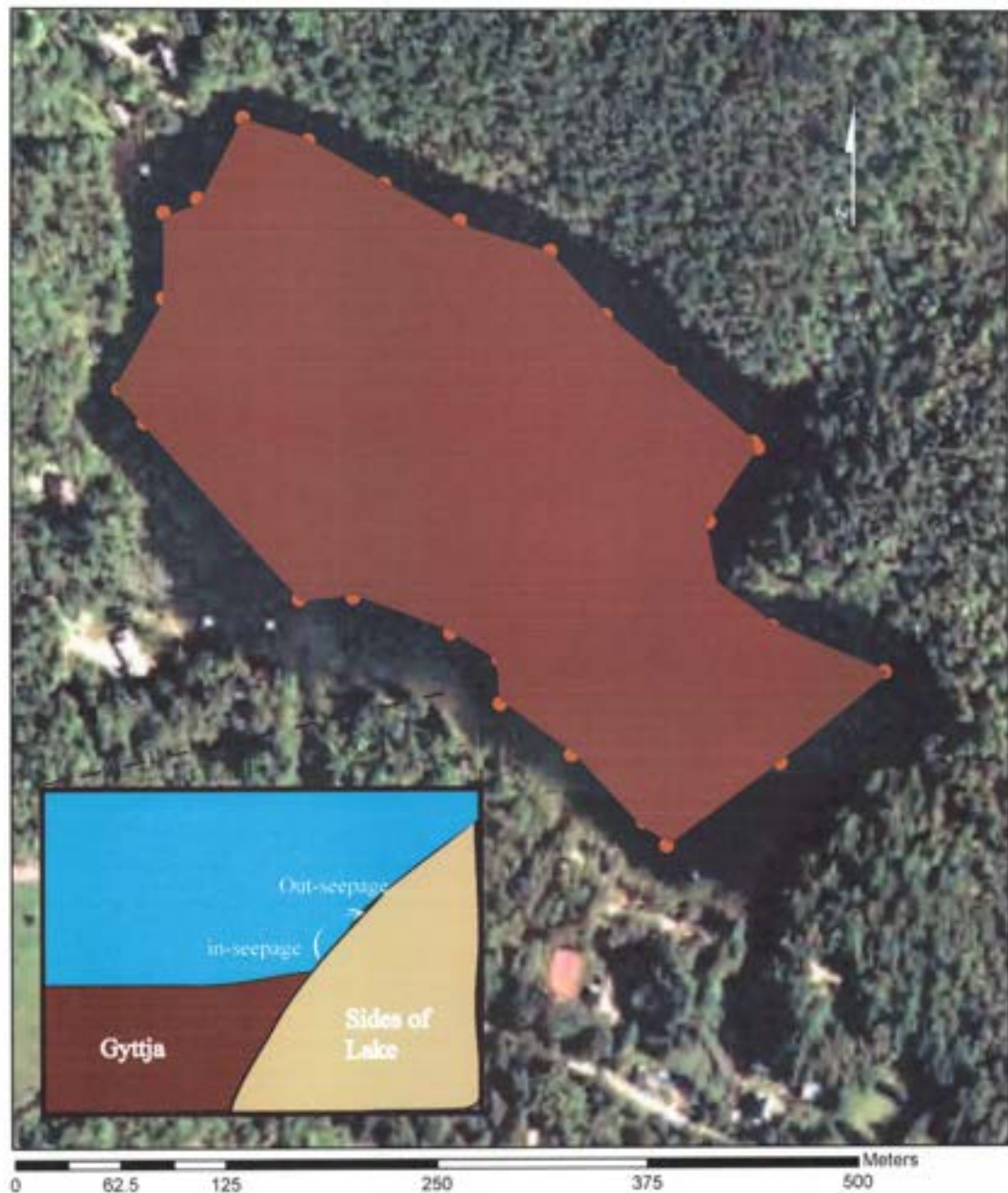
Figure 4-10: Extent of Gyttja Blanket as Inferred from Radargrams. Brown dots represent the edge of the gyttja blanket, as inferred from radargrams. The brown polygon connects those dots and represents the extent of the gyttja. The inset cartoon on the lower left side of that diagram shows the seepage pattern at the interface of the gyttja with the sides of the lake, as inferred by Rosenberry et al. (1999).
