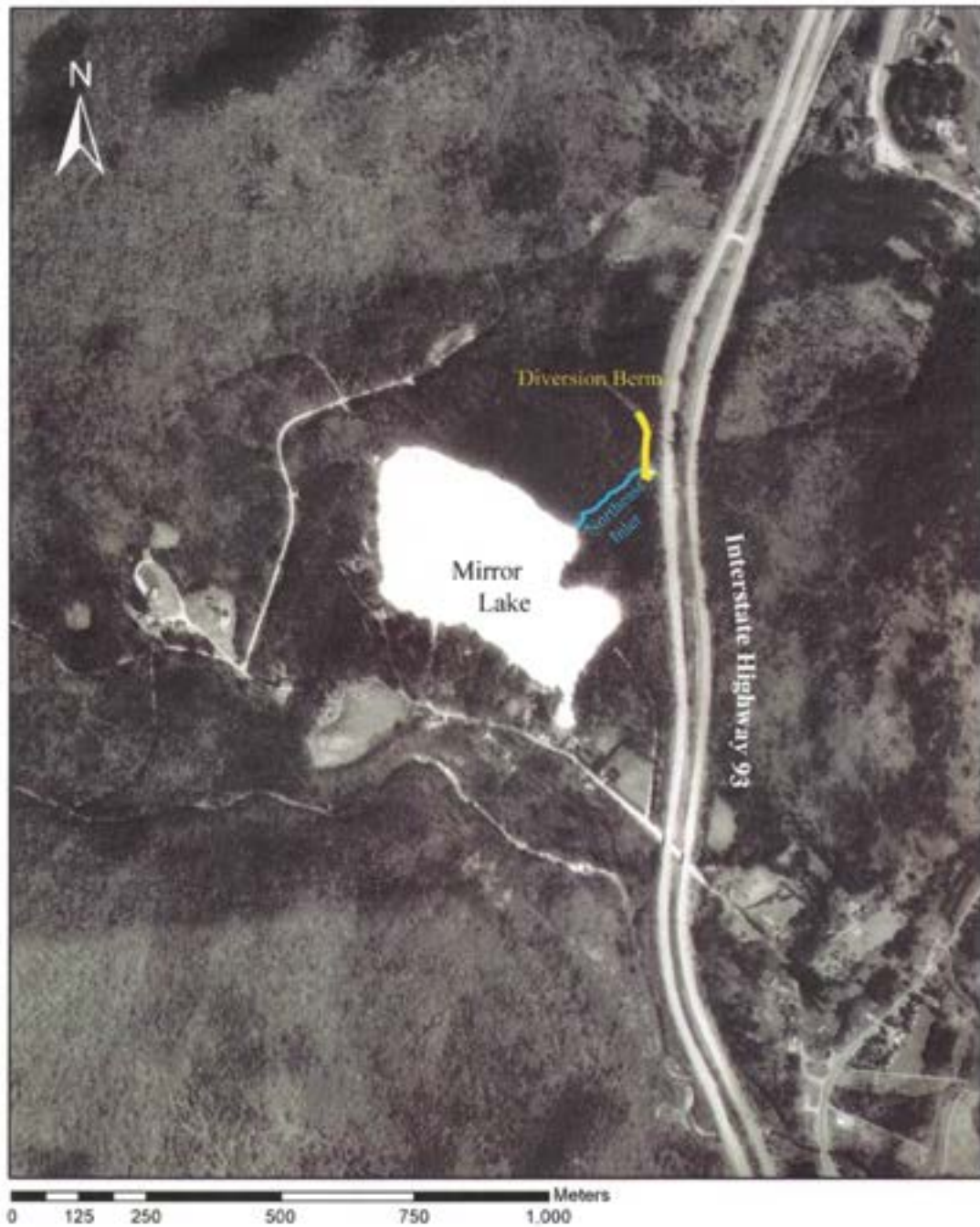
Figure 2-3: Road Salt Contamination at Mirror Lake. Interstate 93 is approximately 100 m from the eastern shore of Mirror Lake at its closest point. Chloride content in Mirror Lake has increased steadily since the 1970's when I-93 was built. A diversion berm (yellow line) pools most highway runoff water and prevents it from entering the Northeast Inlet stream (blue line). Higher-than-baseline chloride concentrations have nonetheless been measured in the Northeast Inlet stream. Orthophoto from Complex Systems Research Center, University of New Hampshire.
