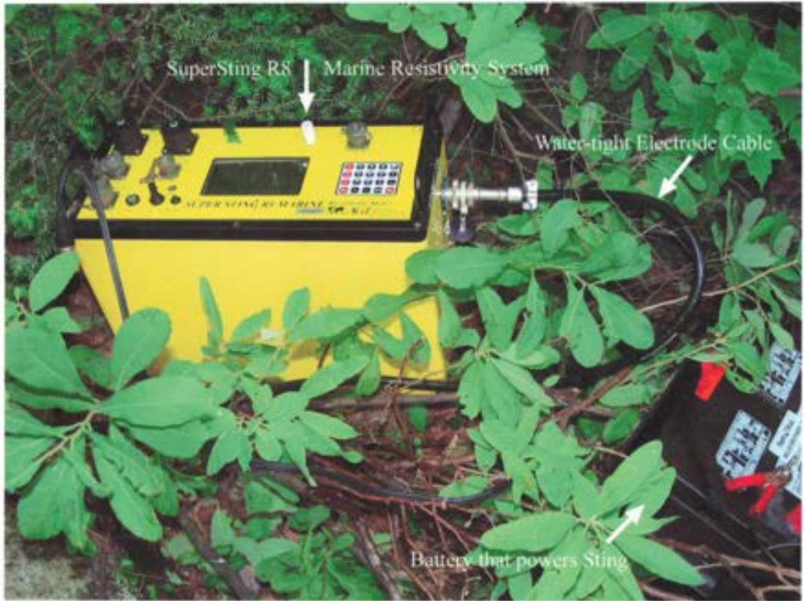
Figure 3-2: SuperSting R8 Marine Resistivity System. SuperSting is shown here on the shore, with electrode cable attached and the battery which powers the SuperSting.
