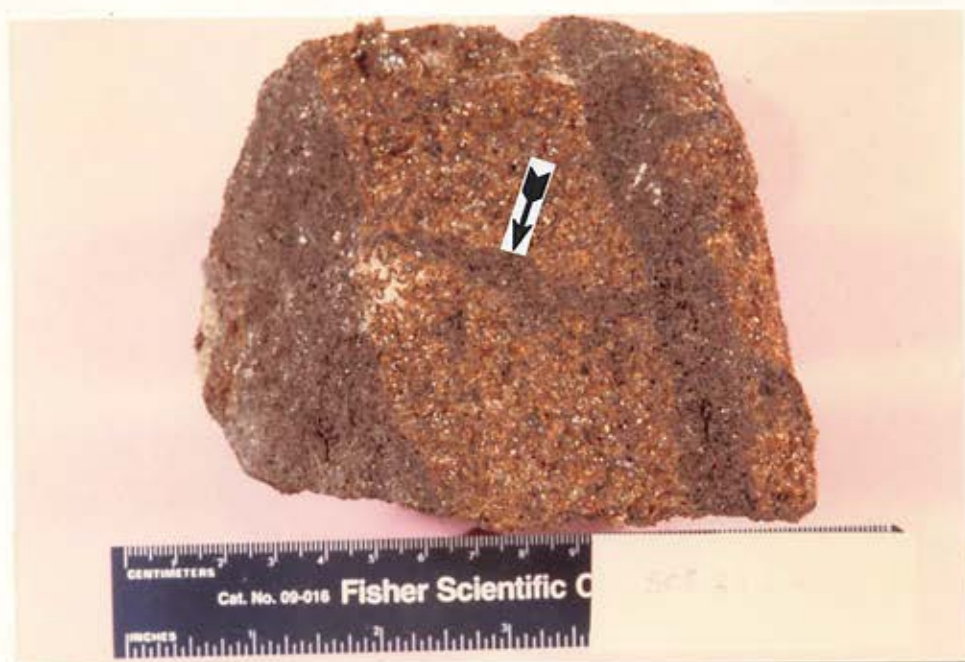
Figure 22. Nodule SCB 383-6: olivine=Fo-76.7; average grain size=1-3 mm, with some large (5 mm) olivine grains; iridescent grain surfaces; friable. Note cross-cutting vein (arrow) connecting two parallel veins.
