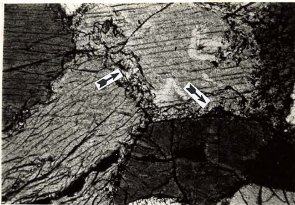
Figure 33. Spongy grain borders (arrows), indicating incipient partial melting. XPL, 2.8 x 2.0 mm.
