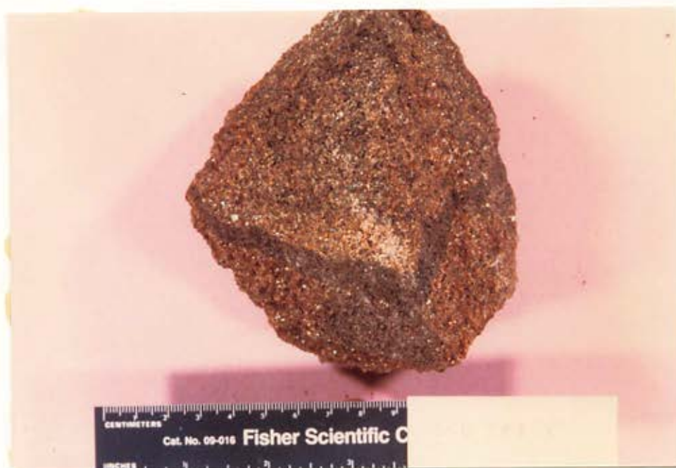
Figure 20. Nodule SCB 383-3: olivine=Fo-76.4; average grain size=1-3 mm; iridescent grain surfaces; friable. Note that lherzolite has a high percentage of dark (CPX, spinel) minerals.
