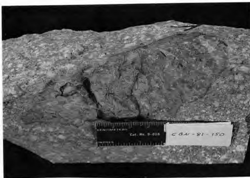
Figure 50 . Altered ultramafic lithology composed of soft hydrous minerals. Specimen shows a bronze-like schiller across large areas of its surface when viewed in sunlight. Deer, et al. (1977, p. 111) state that complete alteration of orthopyroxene to serpentine pseudomorphs can produce specimens with a characteristic bronze-like luster known as "bastite". Ando et al. (1983) noted similar-appearing bastite pseudomorphs after orthopyroxene in harzburgites in ultramafic terrane of the Klamath Mountains, California.
