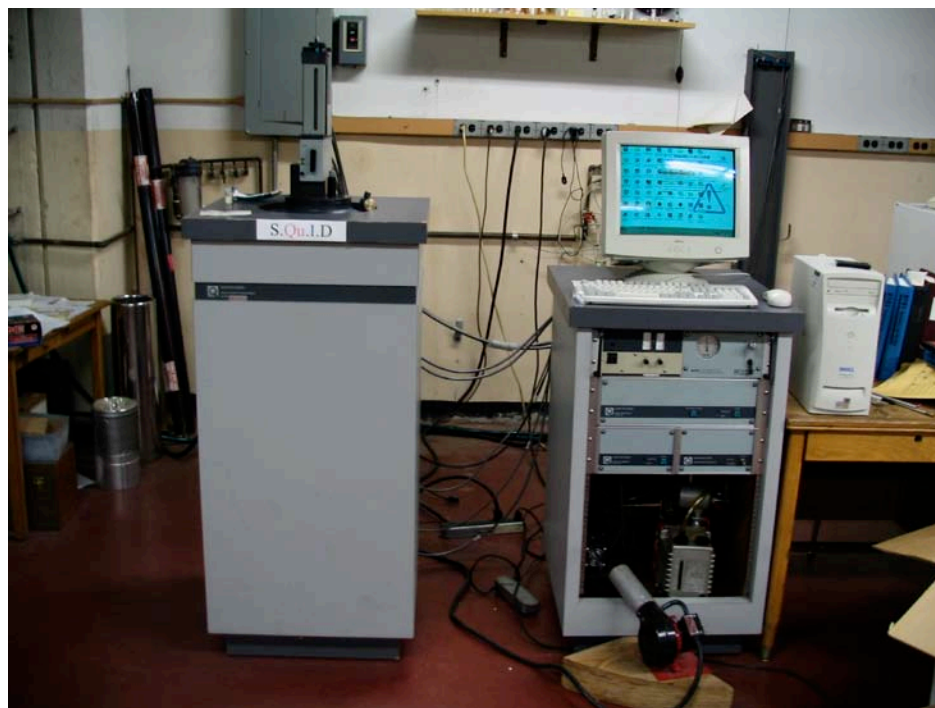
Fig. 3.3. SQUID used in measurements of studied metal organic compounds
