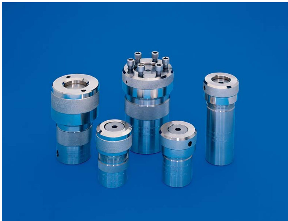
Fig. 3.1. Bombs that are used in hydrothermal route for production of compounds
