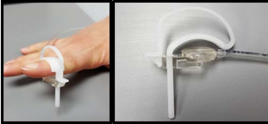
Figure 4. Study 1 Tactile Stimulation. An inflatable membrane mounted in a plastic casing (10 mm diameter; MEG International Services) and surrounding clip placed on the index finger of an adult for Study 1.
