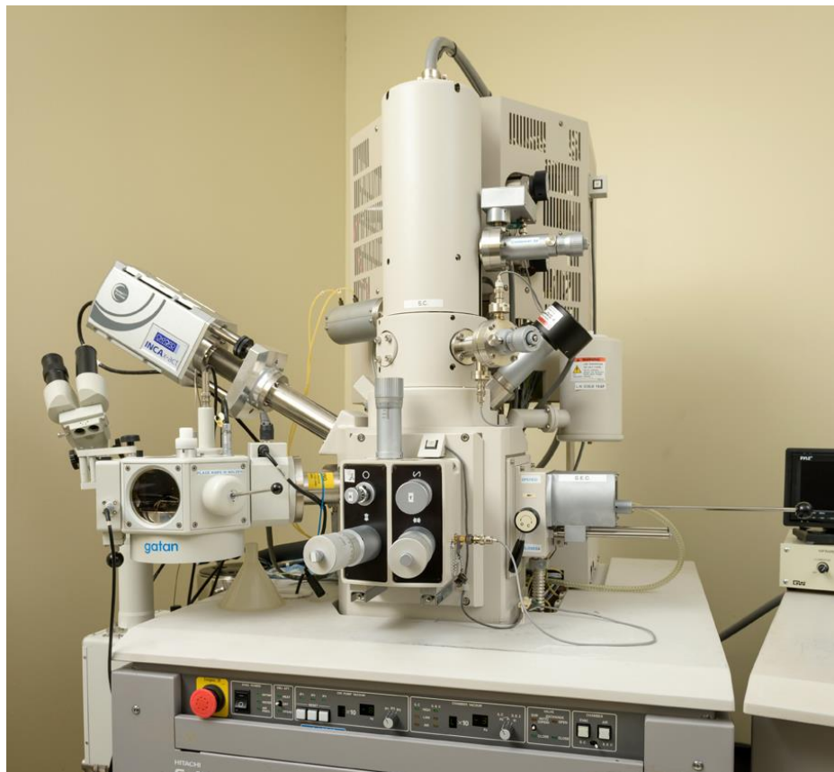
Fig. 5-6. Hitachi S4700 Scanning Electron Microscope with Gatan Alto 2500 cryo-system.
