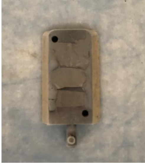
Fig. 5-7. Filters with sample were fixed onto the sample platform, coated with gold platinum.
