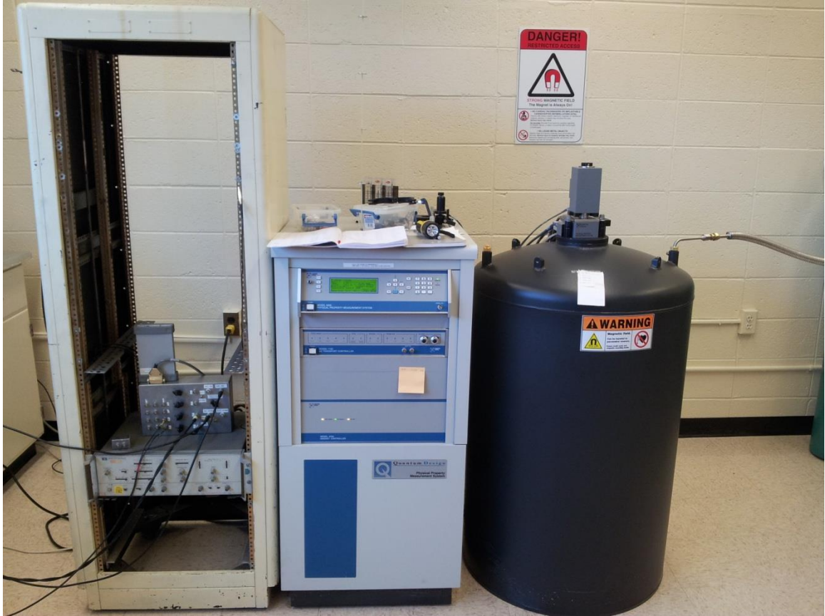
Figure 2.10. Photograph of the Quantum Design PPMS system. Empty rack on the left hand side can be used to interchange measurement electronics.
