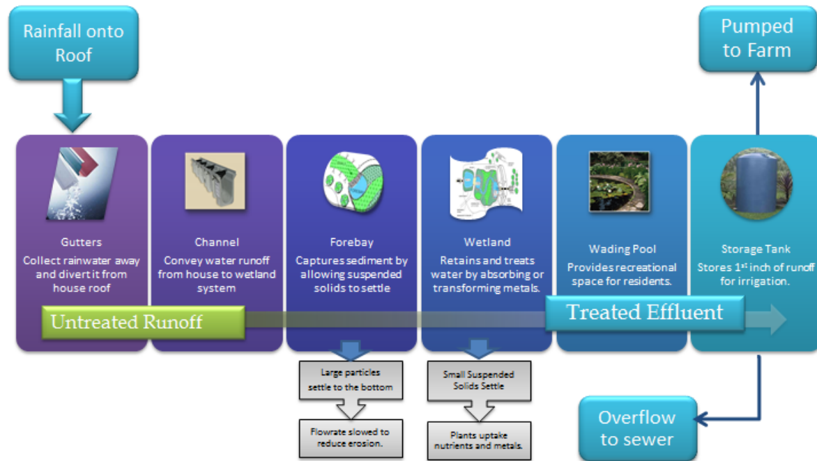
Figure 1: System block diagram illustrating pollutant removal and flow of runoff through the system
