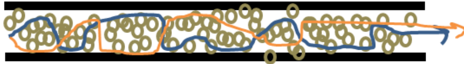
Figure 3-8: Visual illustration of multiple flow paths in a packed column
