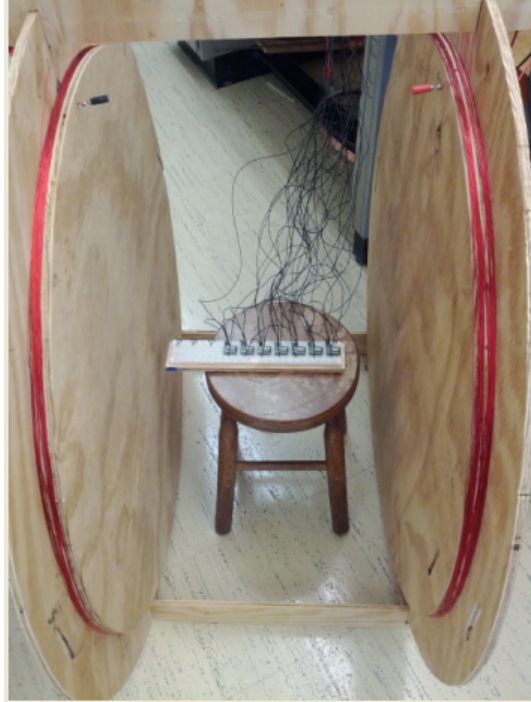
Figure 3.2: Constructed coil with I-beam section for signature creation.
