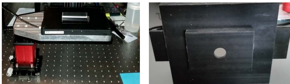
Figure 10. This figure shows the stage of the microscope (left) and the bottom side of the incubation chamber (right). The incubation chamber fits the dimensions of the stage.
