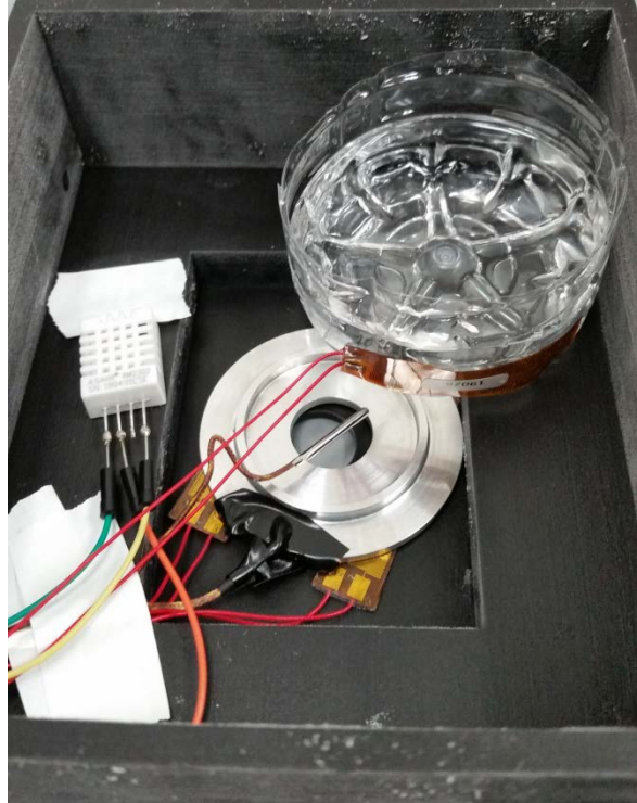
Figure 11. This figure shows the setup for humidity control testing. The water bottle contains water, and there is a heater wrapped around its exterior to heat the water to produce steam. The white cubic object is the humidity sensor. The aluminum ring on the bottom of the chamber is attached to two heaters and to a temperature sensor covered with electrical tape.
