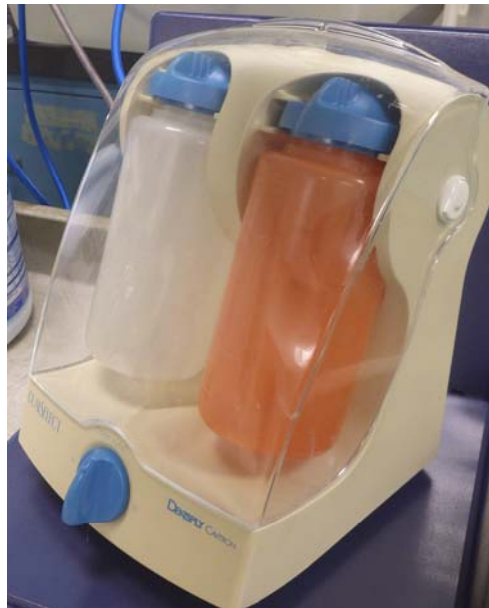
Figure 2. Example of Cavitron Dual Select dispensing system used to deliver distilled water to ultrasonic scaler instruments.
