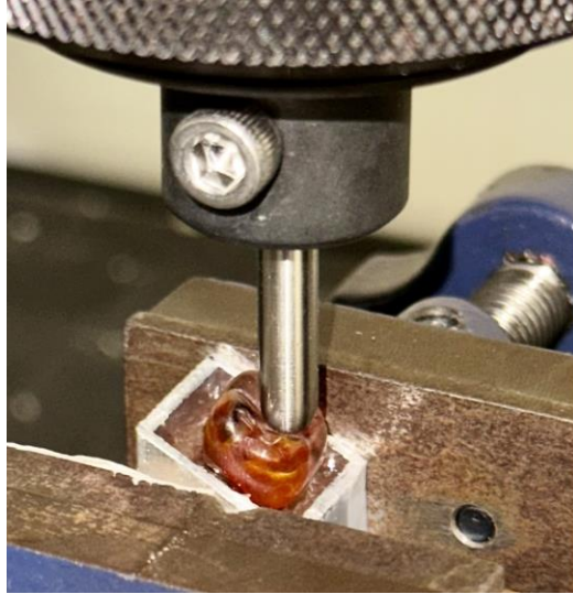
Figure 5. A sample being tested on Instron Universal Testing Machine.
