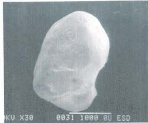
Picture 5: Large rounded iron oxide-dominated particle from profile 3, A-horizon. This particle is more than 1000 \mu\text{m} across.
