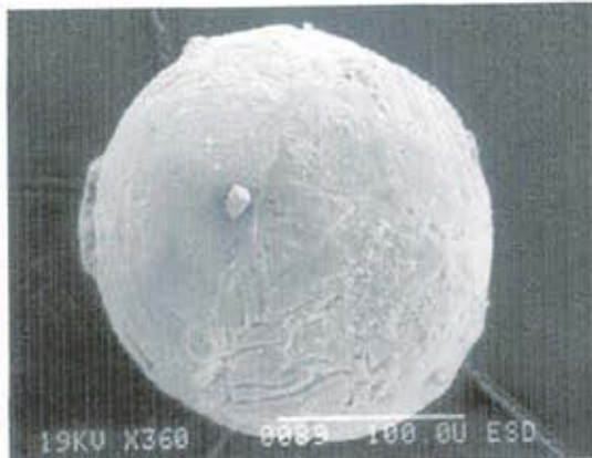
Picture 4: Rounded magnetic particle composed of pure iron oxide based on EDX (Figure A3.3).
