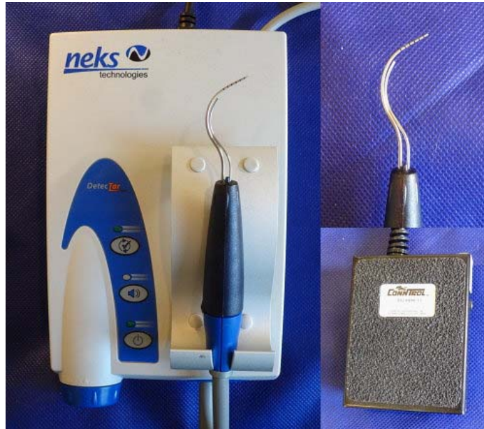
Figure 7. DetecTar device with internal computer housed in unit base (left), with an optical probe embedded within a periodontal probe-like handpiece (upper right), and activated via a foot-depressed switch (lower right).
