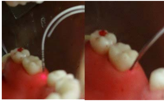
Figure 8. Example of DetecTar periodontal probe-like tip (left) being placed into a subgingival site on typodont model (right).
