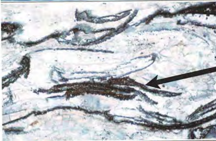
Sample D-3, 10x, reflected light, Poorly washed biosparite.
