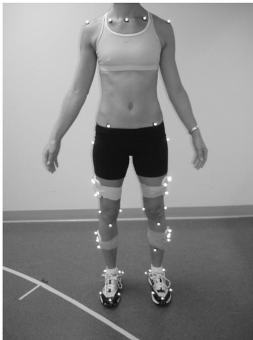
**Figure 3-1. Six degree of freedom marker set utilized to define and track segment motion.**
