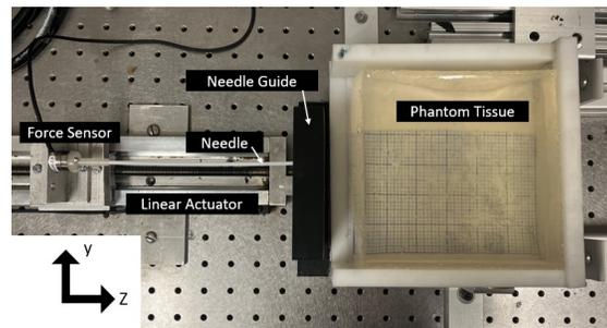
**Figure 2** Experimental Setup for measuring needle insertion and extraction forces
