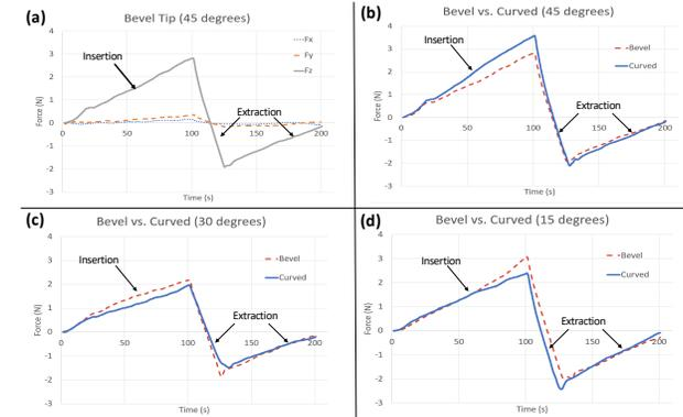
**Figure 3 (a):** Insertion and extraction forces in x, y, and z direction of 45 degrees bevel tip needle. Insertion and extraction forces in z direction of bevel and curved tips of 45 degrees (b), 30 degrees (c), and 15 degrees (d).
