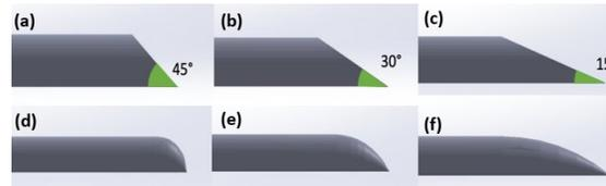
**Figure 1** Different Tip Geometry: Bevel Tip with different angles (a-c), and curved tip (d-f)
