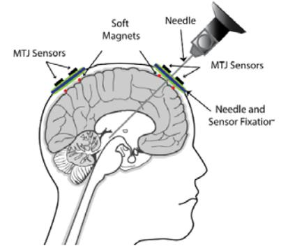
Figure 1: Schematic of implantable brain deformation sensing system.
