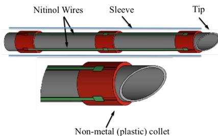
Figure 1. Schematic of smart needle.
