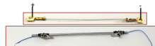
Fig. 4: A Nitinol Actuator (Top), Nitinol Actuator Attached to The Needle Core (Bottom)
