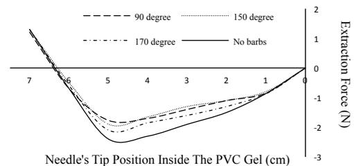
**Figure 2:** The extraction forces of honeybee-inspired needle
