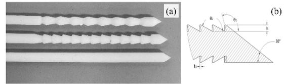
**Figure 1:** 3D Printed honeybee-inspired needles
