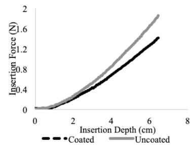
Figure 2: Insertion forces of uncoated and coated needles
