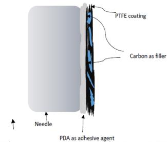
Figure 1: Coating of PDA, PTFE, and Carbon
