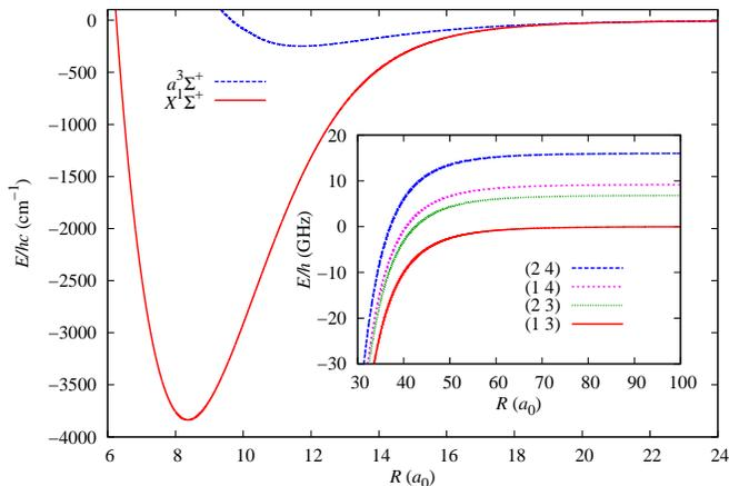
FIG. 1: [Color online.] Molecular potential energy curves  $V_0(R)$  and  $V_1(R)$  for the singlet and triplet states of RbCs correlating with two separated  $^2S_{1/2}$  ground-state atoms. The inset shows an expanded view of the long-range potentials separating to the four different hyperfine thresholds at zero field, labelled by  $(f_{87\text{Rb}}, f_{133\text{Cs}})$ , but no longer by singlet or triplet.
