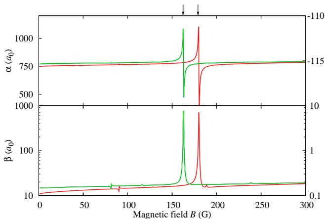
FIG. 10: [Color online.] The real and imaginary parts of the complex scattering length at the Rb  $|2, -1\rangle + \text{Cs } |3, 3\rangle$  threshold, calculated using the final fitted potentials:  $s$ -wave (red, dark gray, left-hand axis) and  $p$ -wave (green, light gray, right-hand axis). The observed resonance positions are shown as arrows at the top of the graph. The three components of the  $p$ -wave scattering length are indistinguishable on this scale.
