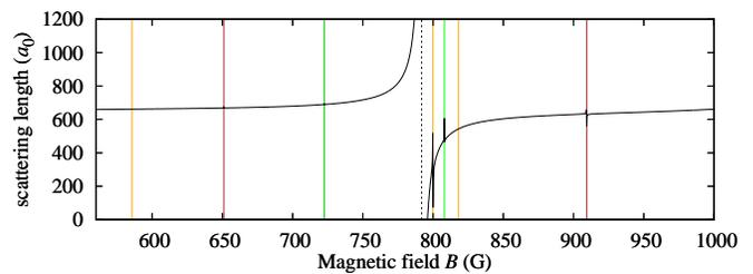
FIG. 11: [Color online.] RbCs scattering length at the  $|1, 1\rangle + |3, 3\rangle$  threshold at fields above 560 G, calculated at  $E = 160$  nK using the final fitted potential. Resonance positions are marked by vertical lines, with the value of  $M_F$  of the corresponding bound state indicated using the same color scheme as in Fig. 8.
