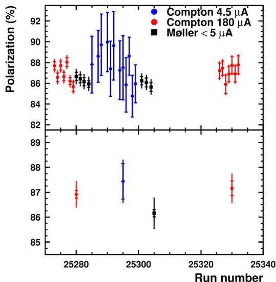
**Fig. 5.** (Top) Polarization measured at 4.5  $\mu\text{A}$  along with neighboring high current runs and the Møller measurements taken at beam currents less than 5  $\mu\text{A}$ . (Bottom) The average of high current and low current Compton and the neighboring Møller measurements.
