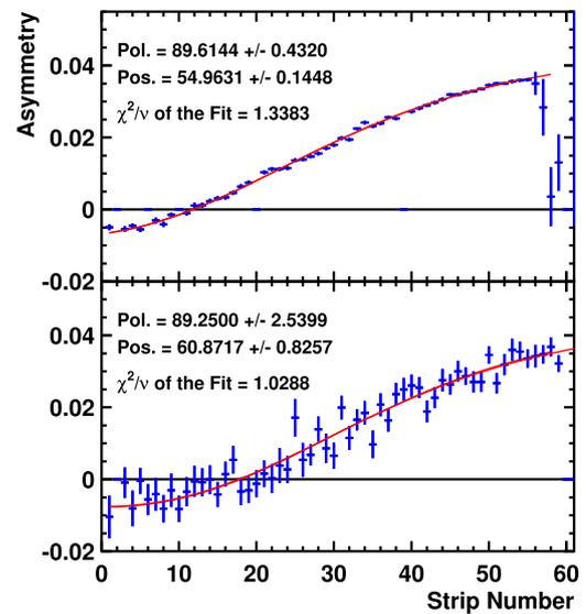
**Fig. 4.** The typical Compton asymmetry (blue) and fit (red) for high current (upper) and low current (lower). The extracted polarization, location of the Compton edge and the  $\chi^2$  per degree of freedom for the fit are also indicated in the figure. (For interpretation of the references to color in this figure legend, the reader is referred to the web version of this article.)
