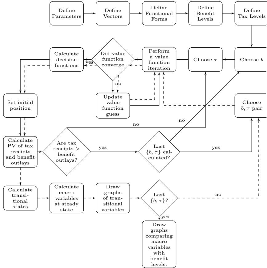
Figure 4.1: A flowchart of the solution algorithm implemented in Matlab. The solid lines indicate the first run through the model where the computer finds the budget balancing tax rate. The dotted lines refer to the second run through the model using the interpolated tax rate found in the first run. The second run is use to find the behavior of the agents.
