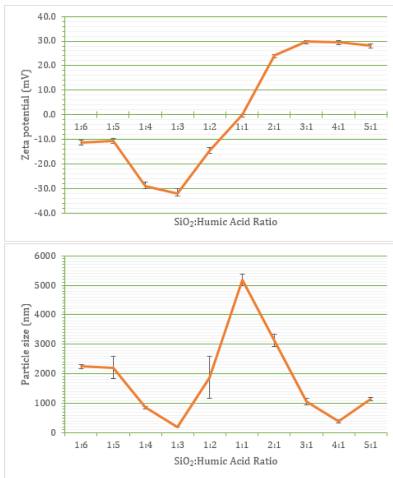
Figure 3.2. Measured zeta potential (top) and particle size (bottom) as a function of the volume ratio of PLL-coated SiO 2 solution to humic acid solution. Error bars represent one standard deviation.
