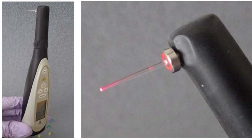
Figure 1. Visible red laser fluorescence-emitting instrument (left) with a periodontal probe-like rigid cylindrical sapphire tip (right).
