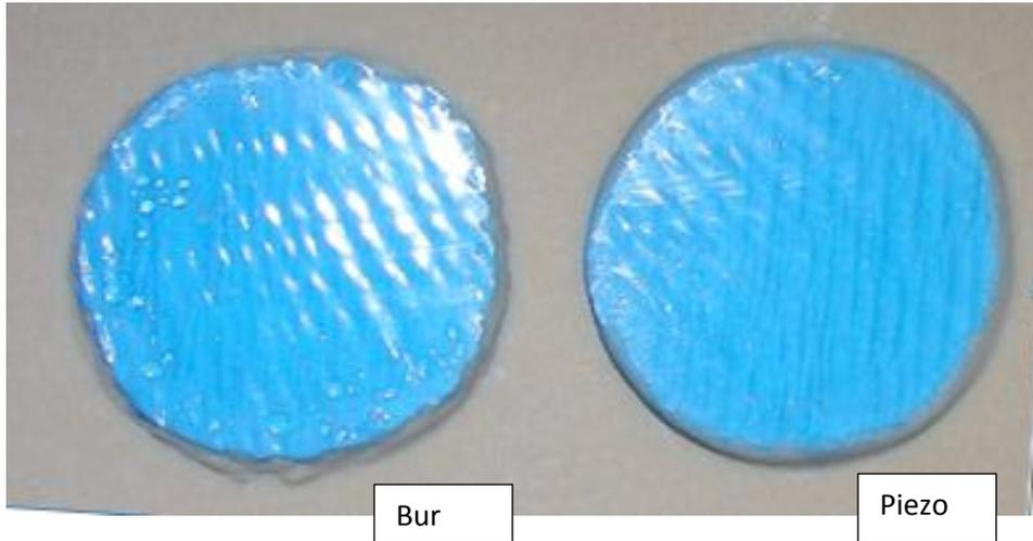
Figure 13. Bur and piezo osteotomies in a polyurethane sheet.
