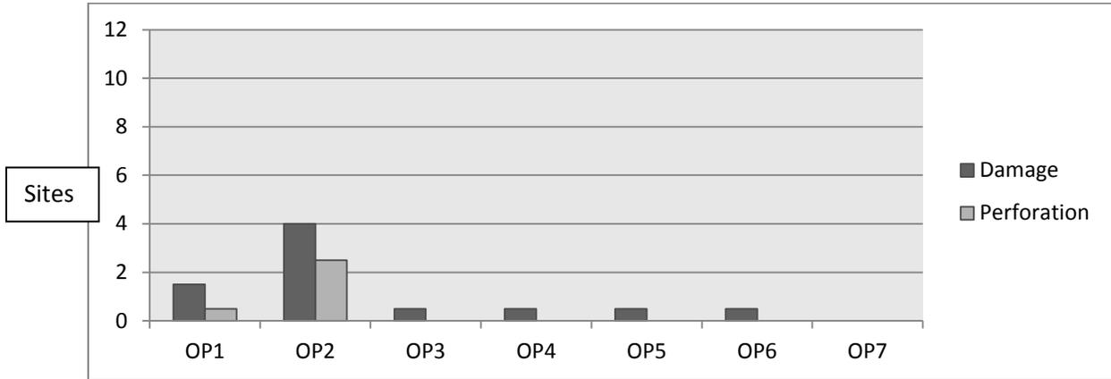
Figure 9. Average number of sites of damage and perforation using piezoelectric instrumentation.
