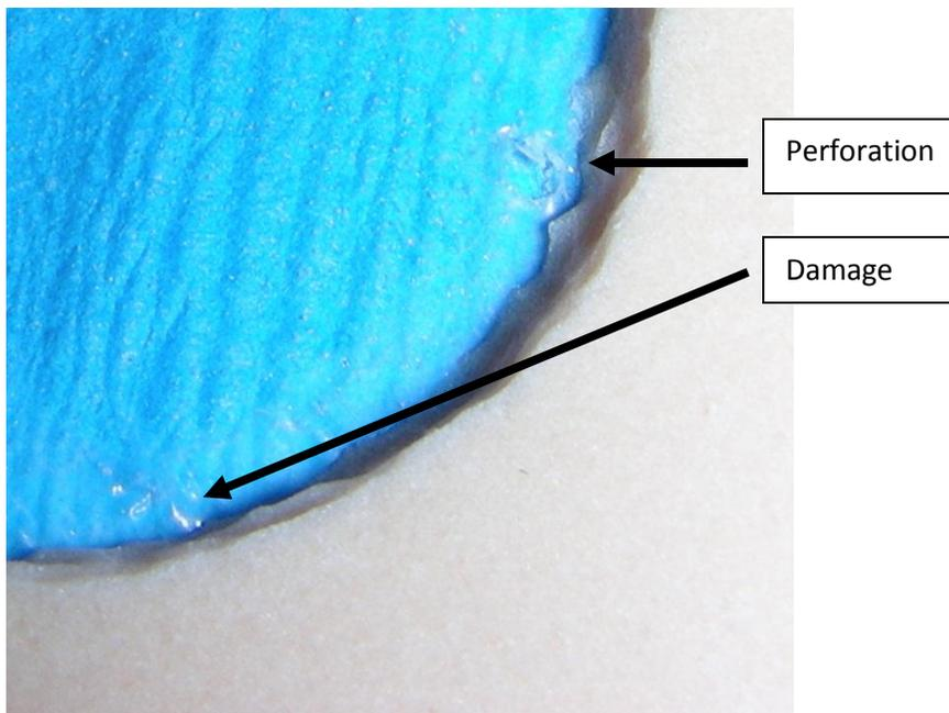
Figure 7. Magnified view of membrane damage and perforation.
