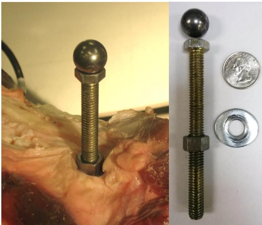
Figure 2.2. Spherical Contact to Machine Actuator. A 3/8" bolt is inserted into the medial condyle of the femur in line with the actuator and system load cell.
